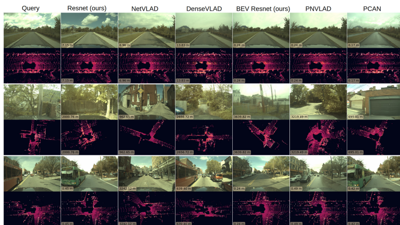
Figure 7.11: Results with occlusion. The first example demonstrates the difficulty in precise image retrieval with few landmarks in the image. The second example shows retrieval failures across the image and LiDAR networks, likely caused by the atypical location and heavy vegetation.
